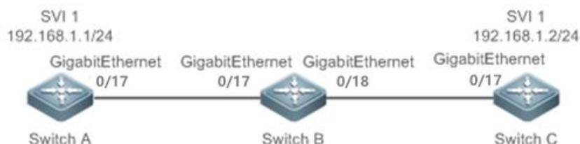
As shown in Figure 1-1 , Switch A, Switch B, and Switch C form a simple L2 data switching network.
