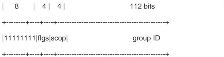
The first byte in the address is all 1s, representing a multicast address.
